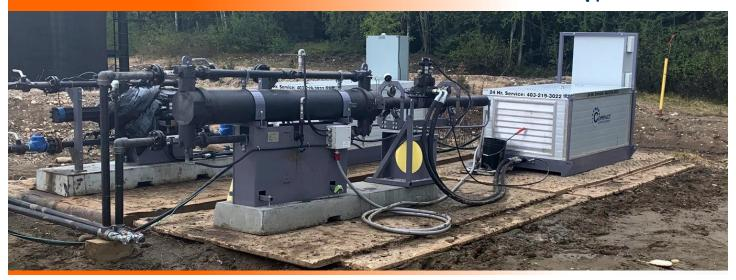
Compact Compression's Multiphase Transfer Pump (MPTP) is directly descended from the ground-breaking HCG Compressor, several of which have been employed in multiphase pumping service. Its principle of operation is very similar to the HCG Compressor with several key enhancements to product design and materials to increase performance, reliability and serviceability for multiphase pumping applications.
